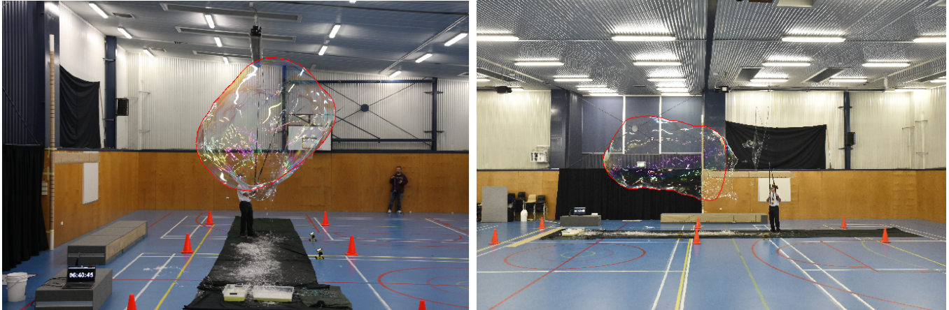
Fig. II.4: Bubble edge selections shown as red lines. Note that the protuberance at the bottom of the end-view image, and the final irregular component of the bubble caused by closure are omitted, thus the model encloses a region smaller than the actual bubble.
